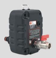
The LT-Sonic is equipped with two main parts. A pulse generator as a Transmitter which is fitting to a fire hydrant, water meter base, or tap, and the hand-held receiver as a geophone to trace buried pipe away from the pulse generator.
